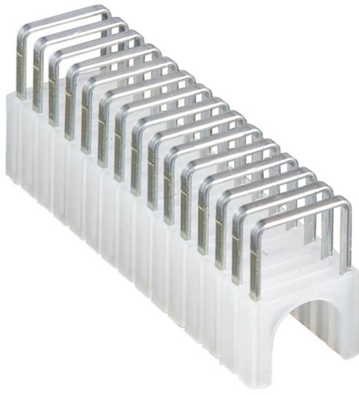
These heavy-duty staples are designed for safe and secure installation of CAT3 and CAT5e data cable, speaker wire and security cable up to 1/4-Inch. For exclusive use with Klein's Loose Cable Stapler (Cat. No. 450-100). These UL listed insulated staples are available in packs of 300.
