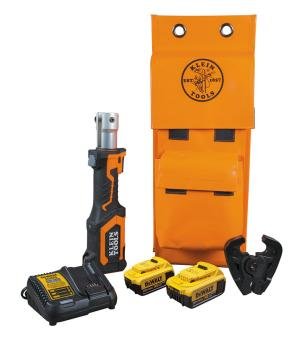
Klein's battery-operated cable crimper is engineered to make linemen's work more efficient by reducing the time and effort needed on the job. Crimps up to 600 MCM copper, 350 MCM aluminum and 477 ACSR cable. 7-ton hydraulic force crimps a larger capacity faster than similar models on the market. Compatible with industry standard W-style dies. Powered by DeWALT 20V lithium-ion batteries. Includes cutting jaw, two 4 Ah batteries, charger and bag.
