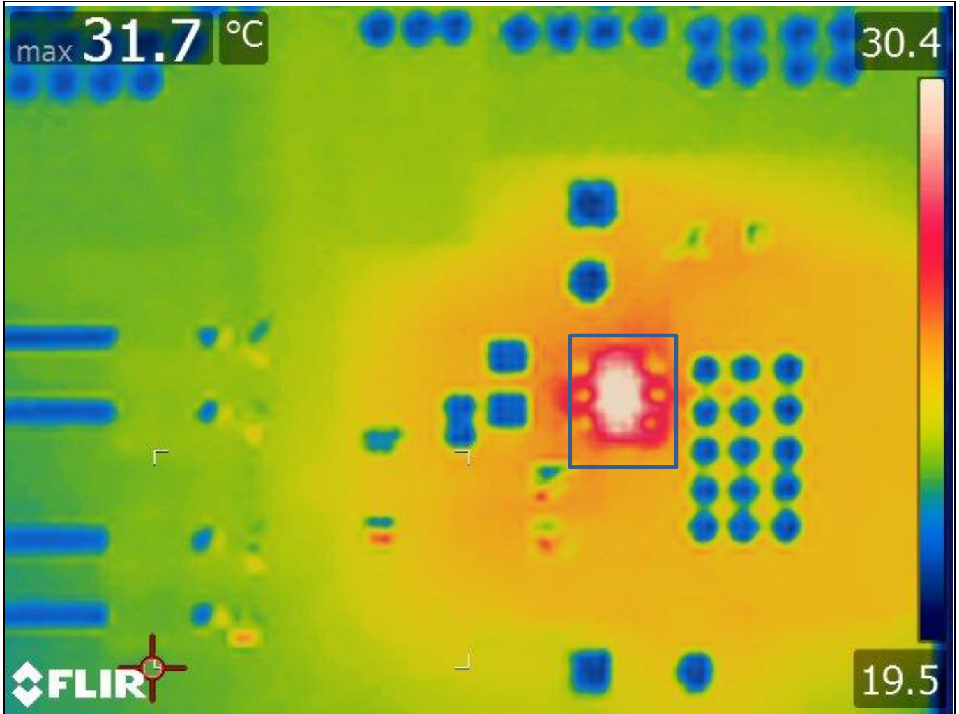
Figure 13 Thermal photo ( V_{IN} = 24\text{ V} , R_{set} = 60.4\text{ k}\Omega , I_{LED} = 15\text{ mA} , T_A = 25^\circ\text{C} )
