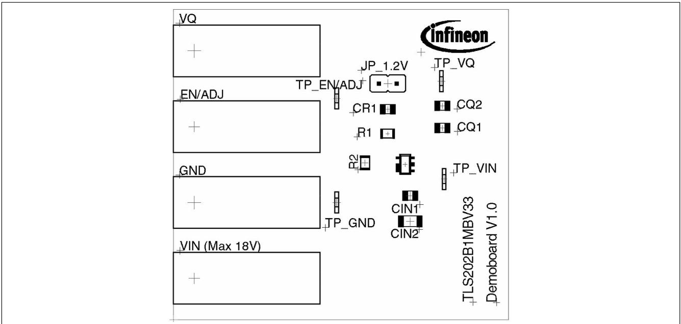
Figure 6 Top Layer components of TLS202B1 Demonstration Board
