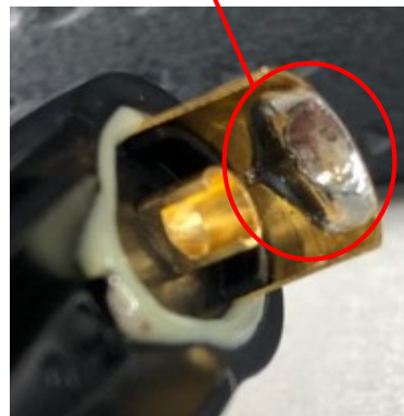
Solder to guarantee contact between Reed and Sleeve
