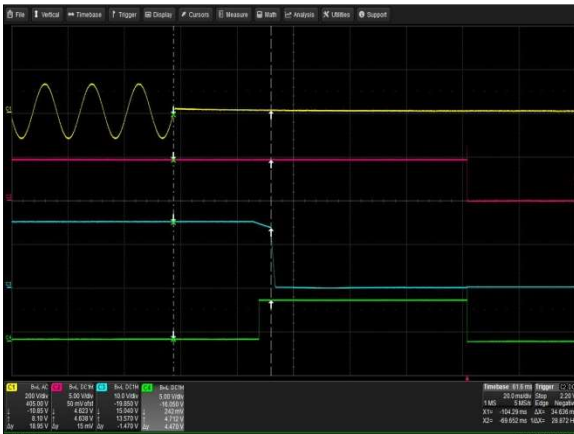
Figure 14: LCM600N Hold-up Time – V_{in} = 90V_{ac} / 63Hz / 0^\circ Full Load: I_o = 40A (15V), I_{SB} = 2A (5V) Ch 1: AC Mains Ch 2: VSB Ch 3: Vo Ch 4: POWER GOOD
