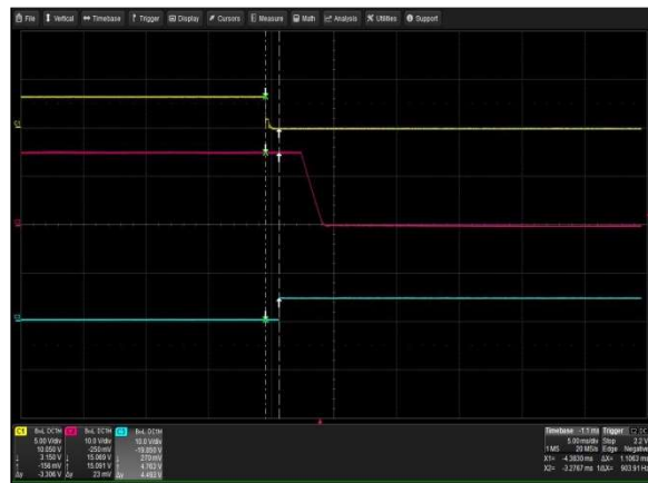
Figure 17: LCM600N Turn Off Characteristic via INH_EN Full Load: I_o = 40A (15V), I_{SB} = 2A (5V) Ch 1: INH_EN Ch 2: Vo Ch 3: POWER GOOD
