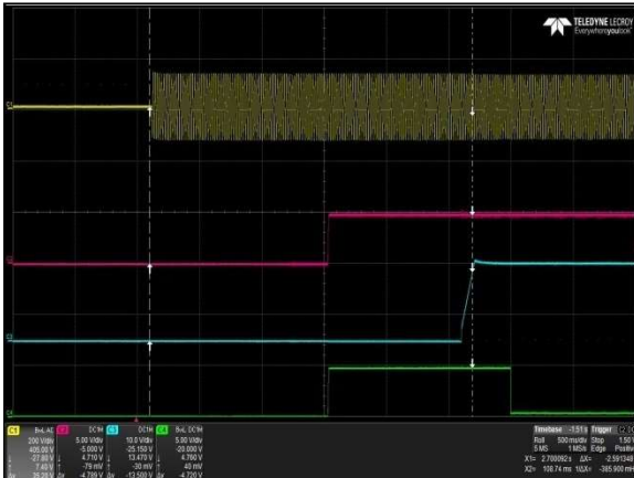
Figure 12: LCM600N Turn-on delay via AC mains – V_{in} = 90V_{ac} Full Load: I_o = 40A (15V), I_{SB} = 2A (5V) Ch 1: AC Mains Ch 2: VSB Ch 3: Vo Ch 4: POWER GOOD
