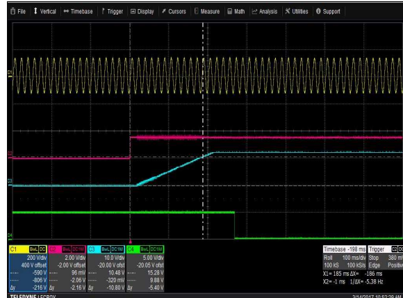
Figure 2: LCM300L Turn-on delay via INH_EN – Vin = 90Vac Full Load: Io = 25A (12V), ISB = 2A (5V) Ch 1: AC Mains Ch 2: INH_EN Ch 3: Vo Ch 4: G_DCOK_C
