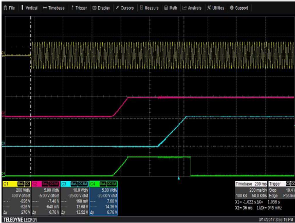
Figure 12: LCM300N Turn-on delay via AC mains – Vin = 90Vac Full Load: Io = 20A (15V), ISB = 2A (5V) Ch 1: AC Mains Ch 2: VSB Ch 3: Vo Ch 4: G_DCOK_C
