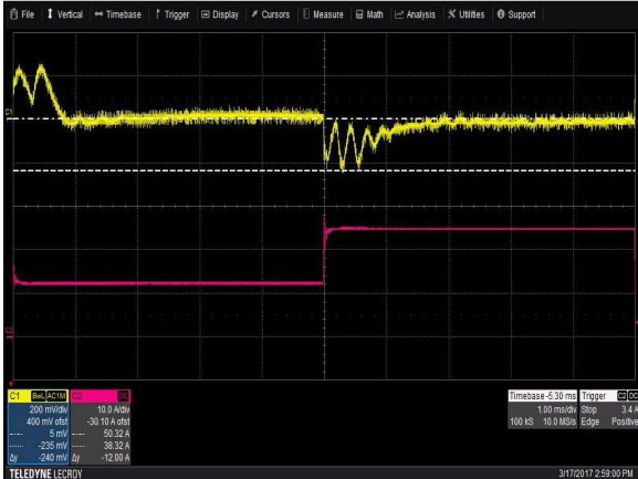
Figure 7: LCM300L Transient Response – Vo Deviation (low to high) 50% to 100% load change, 1A/ \mu S slew rate, Vin = 230Vac Ch 1: Vo Ch 2: Io
