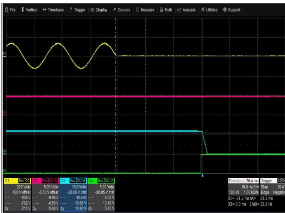
Figure 3: LCM300L Hold-up Time – Vin = 90Vac / 47Hz Full Load: Io = 25A (12V), ISB = 2A (5V) Ch 1: AC Mains Ch 2: VSB Ch 3: Vo Ch 4: G_DCOK_C
