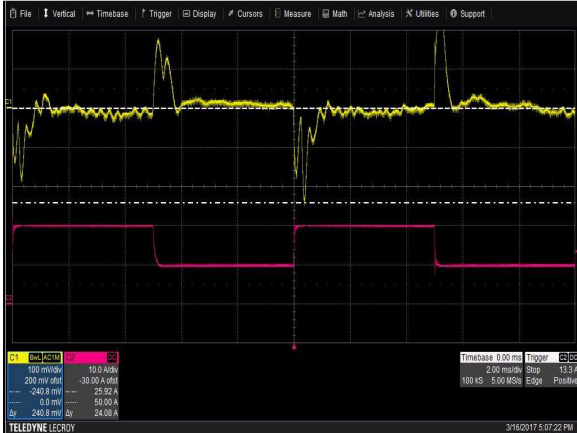
Figure 18: LCM300N Transient Response – Vo Deviation (low to high) 50% to 100% load change, 1A/ \mu S slew rate, Vin = 230Vac Ch 1: Vo Ch 2: Io
