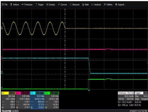
Figure 14: LCM300N Hold-up Time – Vin = 90Vac / 47Hz Full Load: Io = 20A (15V), ISB = 2A (5V) Ch 1: AC Mains Ch 2: VSB Ch 3: Vo Ch 4: G_DCOK_C
