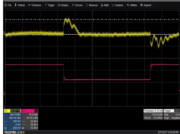
Figure 8: LCM300L Transient Response – Vo Deviation (high to low) 100% to 50% load change, 1A/ \mu S slew rate, Vin = 230Vac Ch 1: Vo Ch 2: Io
