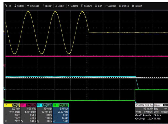
Figure 4: LCM300L Hold-up time – Vin = 264Vac / 60Hz Full Load: Io = 25A (12V), ISB = 2A (5V) Ch 1: AC Mains Ch 2: VSB Ch 3: Vo Ch 4: G_DCOK_C
