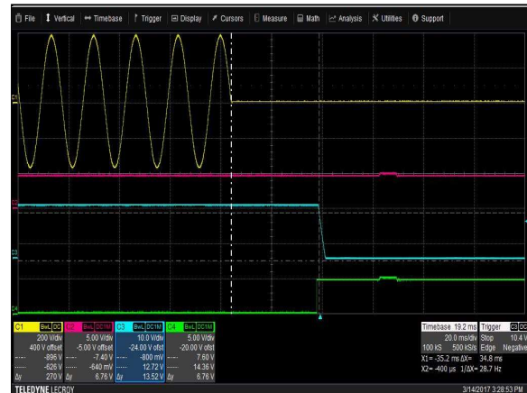
Figure 15: LCM300N Hold-up time – Vin = 264Vac / 60Hz Full Load: Io = 20A (15V), ISB = 2A (5V) Ch 1: AC Mains Ch 2: VSB Ch 3: Vo Ch 4: G_DCOK_C
