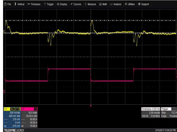
Figure 19: LCM300N Transient Response – Vo Deviation (high to low) 100% to 50% load change, 1A/ \mu S slew rate, Vin = 230Vac Ch 1: Vo Ch 2: Io
