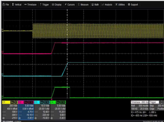
Figure 1: LCM300L Turn-on delay via AC mains – Vin = 90Vac Full Load: Io = 25A (12V), ISB = 2A (5V) Ch 1: AC Mains Ch 2: VSB Ch 3: Vo Ch 4: G_DCOK_C
