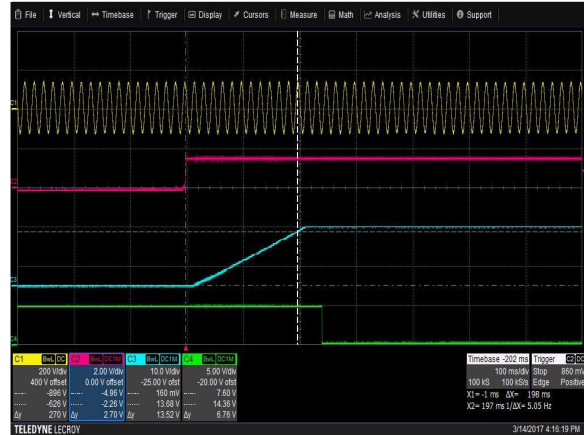
Figure 13: LCM300N Turn-on delay via INH_EN – Vin = 90Vac Full Load: Io = 20A (15V), ISB = 2A (5V) Ch 1: AC Mains Ch 2: INH_EN Ch 3: Vo Ch 4: G_DCOK_C
