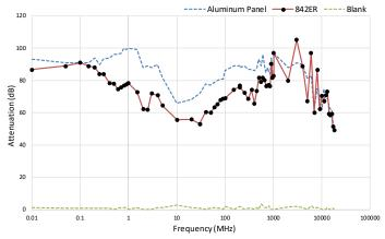
Test performed with a two-coat thickness.
