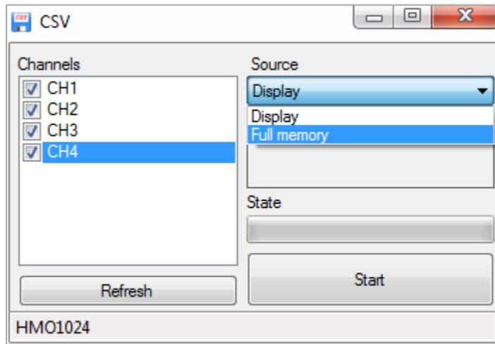
Depending on the selected source and channel, reading the waveform data may require a lot of time. Storage requirements will increase by 8, as well as the transferable data stream, if the waveform data is converted from an internally used number format to an ASCII format for a CSV file, for instance. These large amounts of data will require extended waiting periods since the R&S®HMO oscilloscopes do not have data logging capacities.
