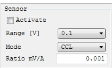
selected sensor mode. In sensor mode “EXTS”, “Resistance” is used to enter the value of the externally connected shunt in ohms. Once the shunt value is entered, all measured values (current, power and values derived from these) can be calculated correctly and displayed. Manual calculations are no longer necessary. The data from the external shunt is converted to the correct measured values internally.
