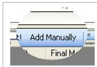
If you wish to include a frequency in the re-measurement that was not detected in the peak value detection, you can click on "Add Manually" to generate an entry in the list. In this case, the value is entered manually. The entry is shown in the peak list with the comment "Manual". Therefore, any number of locations in the spectrum can be marked and measured.
