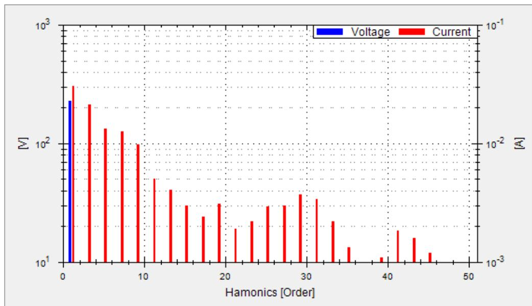
In the display mode „Harmonics“, FFT is used to calculate the RMS value and phase angle of the harmonics. This includes a calculation of the first 50 harmonics (100kHz max.). Instead of the total RMS value, the bar graph display shows the voltage level (Blue) and the current level (Red) of the individual harmonics.
