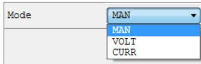
Via the drop-down menu „Mode“ in the left menu section the trigger can be set to „VOLT“ (voltage trace), „CURR“ (current trace) or “MAN” (manual trigger selection).
