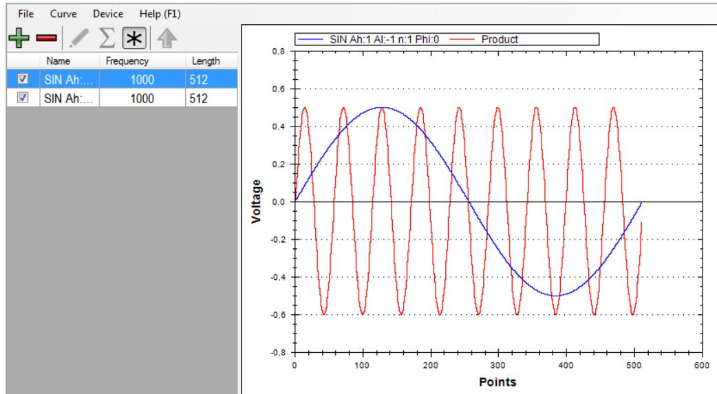
If one waveform is shorter than the other, the missing points will be filled with the value 1.
