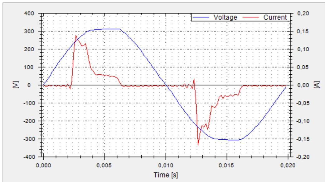
The “Waveform” display mode can be used to display the voltage (**blue**) and current (**red**) simultaneously as a trace on the screen (hardware-based triggering). Exactly one signal period is displayed in the measurement diagram and automatically scaled to the measuring range (100kHz max.).
