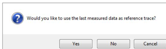
After performing a pre-measurement with a desired detector, you can perform an additional pre-measurement with another detector (if required). You can include the previous measurement as reference curve.
