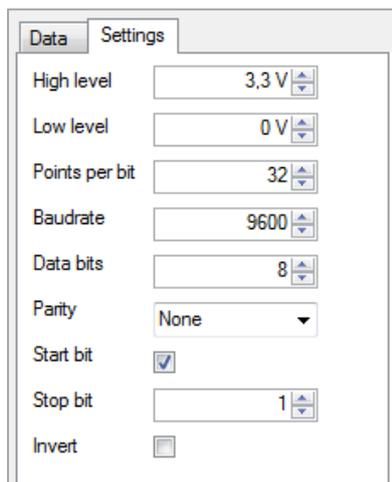
The second tab allows you to select the RS-232 settings. You can use the high and low levels to select the amplitude and the offset here. The options “Points per bit” and “Baudrate” define the number of points for the period. In this case, the option “Points” on the upper right margin of the screen cannot be adjusted.
