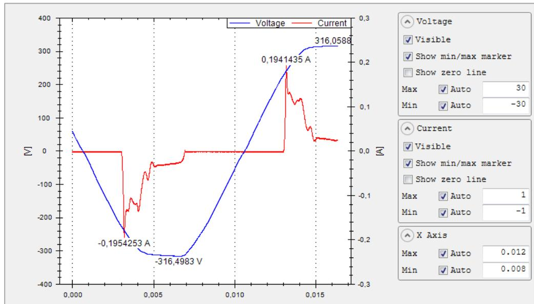
“Inrush” display mode uses an internal hardware buffer to trigger acquisition of a rare event and to output it to the display (similar to the single shot function found on oscilloscopes). This might be used to acquire inrush currents on loads, for example. After an event occurs, the current and voltage trends are acquired.
