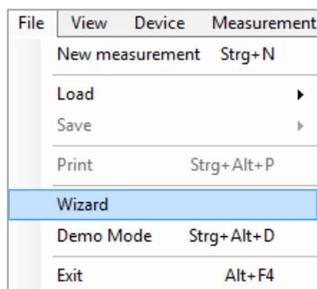
Use "File" → "Wizard" to start the internal software wizard which guides you through all required steps of the measurement setup. You can either select the settings for amplifier/attenuator, transducer and limit lines from the list or use the option "New" to enter them with the CSV Editor. The measurement settings are entered manually.
