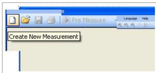
Use “Create new measurement“, Wizard (“File“ → “Wizard“ or “File“ → “New measurement“ to create a new test set configuration. This opens the Setup window where you can select all necessary settings. Settings for transducer, amplifier/attenuator and limit lines are defined in advance based on the previously described procedure.
