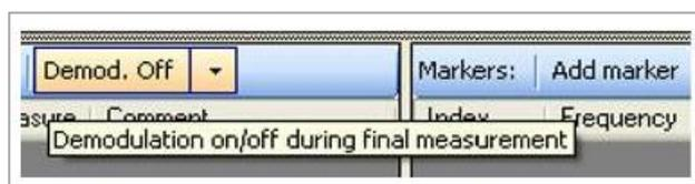
In addition, it is possible to activate the demodulator during the re-measurement for each frequency of the measurement receiver for a specific amount of time
