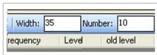
You can determine the values for "Width" and "Number" of the peak value detection in the lower left of the measurement window ("peak detector"). "Number" indicates the amount of the peaks to be detected and "Width" indicates the
