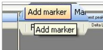
In addition to the peak value detection, you can also select additional markers. You can insert any number of marker values by double-clicking the measurement curve or by clicking “Add marker”. For each entry in the marker list, an identifier with a corresponding number is added to the signal section. Use the function “Marker to Highest peak”
