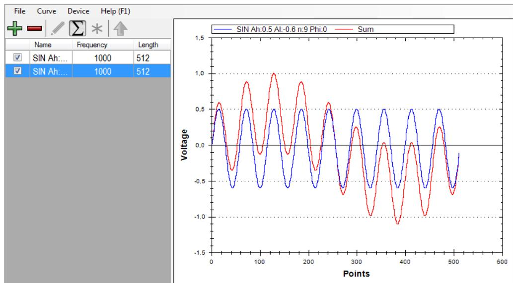
If one waveform is shorter than the other, the missing points will be filled with the value **0**.
