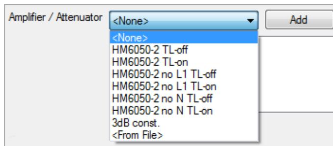
The following correction factors for the HM6050-2 are integrated in the software (please refer to the HM6050-2 data sheet „Insertion Loss“):
