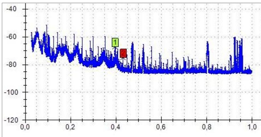
The “Delta Limit“ is the distance of the level (at the corresponding location in the spectrum) to the set limit. A negative value indicates that the level is below the limit. Is the level above the limit, the value is positive and will be displayed in a red font.
