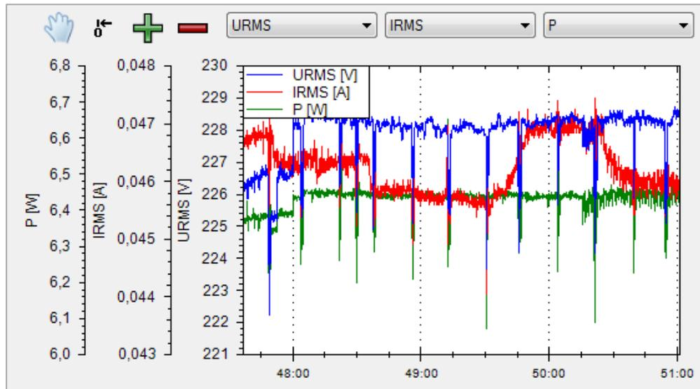
Using display mode “Trendchart” current or voltage values can be displayed as a signal profile (similar to the roll mode in an oscilloscope). Compared to the “trendchart” display mode on the instrument the “Trendchart” display mode via power analyzer software is used to show up to three selected values over time simultaneously.
