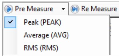
**PEAK:** The peak value detector shows the highest level during the selected measurement time
