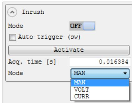
The „Inrush“ mode will be activated (scroll bar ON) resp. deactivated (scroll bar OFF) via “Inrush” menu and function “Mode”. The trace display does not update dynamically. Instead, it must be updated manually by pressing button “Activate”. The trace is updated each time the button is pressed (single shot).
