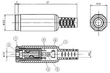
Material Description Number Material Finish Thickness Body PA 1 \_ 2 Sleeve BSR \_ Ni 3 Contact A 0.25 4 Contact B Au PBS - EH 0.3 5 Contact C Ni 6 Contact D 0.3 7 Cap PE -\_
