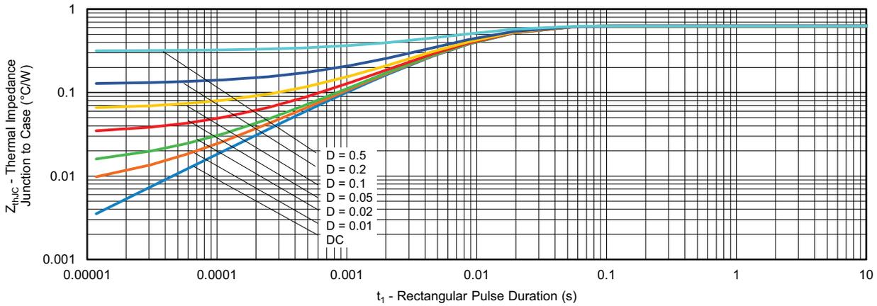
Fig. 5 - Typical Thermal Impedance  $Z_{thJC}$  Characteristics, per leg
