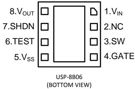
\*The dissipation pad for the USP-8B06 package should be solder-plated in recommended mount pattern and metal masking so as to enhance mounting strength and heat release.
