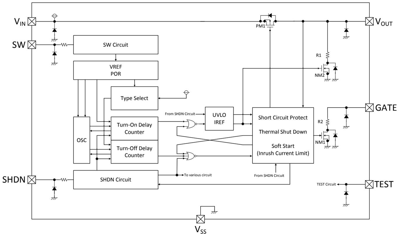
\*Diodes inside the circuit are an ESD protection diodes and a parasitic diodes.
