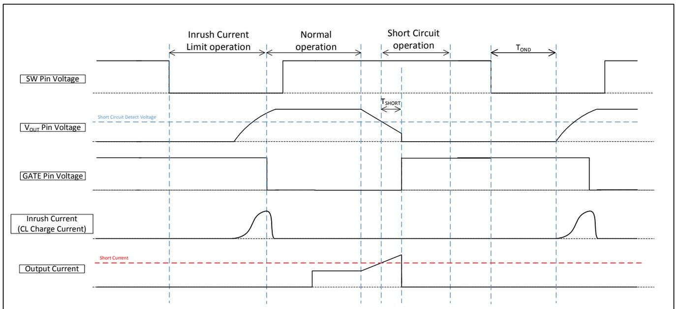
Fig.10 Inrush current limit and short circuit protection
