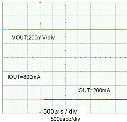
$V_{IN}=5.0V$ ,  $V_{OUT}=3.3V$ , MODE/SYNC=0V (PWM/PFM automatic switching control)
