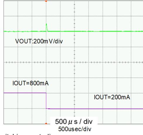
$V_{IN}=5.0V$ ,  $V_{OUT}=3.3V$ ,  $MODE/SYNC=V_{IN}$  (PWM/PFM automatic switching control);
