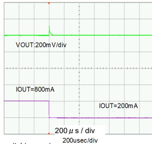
$V_{IN}=5.0V$ ,  $V_{OUT}=1.5V$ , MODE/SYNC= $V_{IN}$  (PWM/PFM automatic switching control),  $C=0V$ ,  $T_{opr}=25^\circ C$
