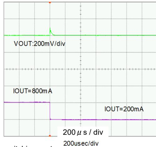
$V_{IN}=5.0V$ ,  $V_{OUT}=1.5V$ ,  $C=0V$  (PWM/PFM automatic switching control)
