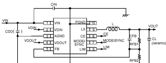
(\*1) A capacitor of 2200pF~ $0.1\mu F$  is recommended to place at the  $C_{DD}$  between the AGND pin and the  $V_{IN}$  pin.
