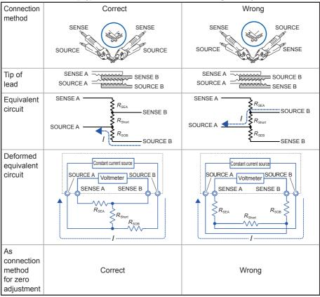
Table 2: Clip type lead connection methods used during zero adjustment
