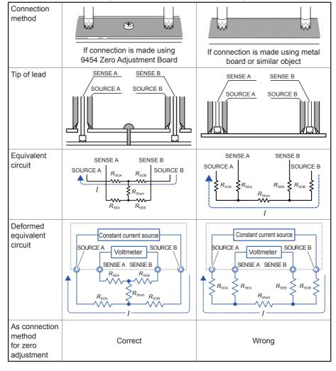
Table 3: Pin type lead connection methods in zero adjustment
