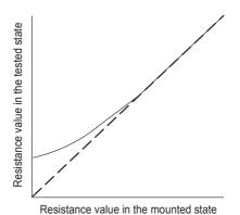
Fig. 17 Difference between the mounted state and tested state
