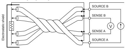
Fig. 3 Noise reduction for the instrument
