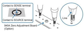
For the pin on the SENSE side, a line is attached to the base section.
