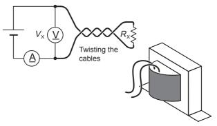
Fig. 2 Twisting cables near a high current line
