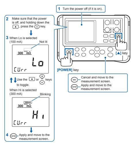
When measurement is performed with the 300 mA measurement current, the 300 mA indicator lights up.
