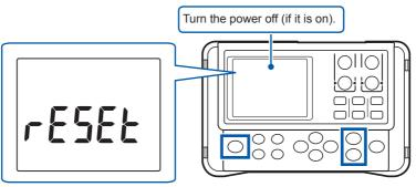
System reset: Resets all settings other than the clock settings, including the panel data and saved measurement data, to the factory defaults.
