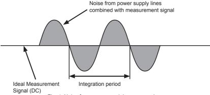
Fig. 4. Noise from a commercial power supply
