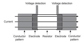
Fig. 14 Current flow in the mounted state
