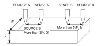
Fig. 9 Probe positions on wider/thicker measurement target
