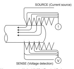
Fig. 6 Measurement with the L2107 4-Terminal Probe
