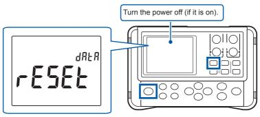
Reset (to reset the current measurement conditions): Resets data and settings other than the
