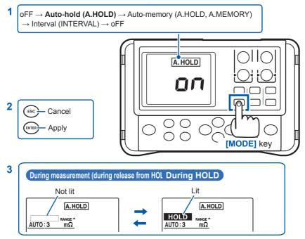
Release the test leads from the measurement target and contact the leads to the target again. The HOLD is released. You can also release the HOLD by changing the range or pressing the [ESC] key.
