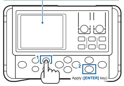
Panel load setting ([PANEL] key) Panel save setting (Press and hold the [PANEL] (SAVE/ **CLEAR)** key)
