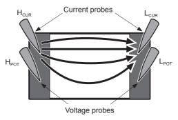
Fig. 16 Current flow in the mounted state
