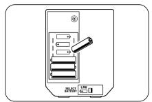
Turn the battery selector switch to LR6.
