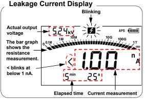
3.2.5 "Switching to Leakage Current Indication" (page 74)
