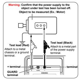
Clip the alligator clip at the end of each test lead to the object under test.
