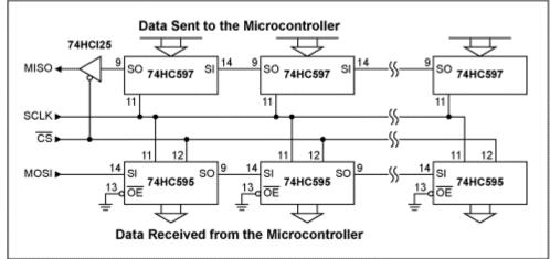
When driven by an SPI master, this circuit converts the SPI signals to steady outputs for easy probing. BACK TO OUESTIONS
