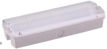
The new Emergency Maintained / Non-Maintained LED Bulkhead has a single 3.5W LED strip that produces 150 lumens in standard and 110 lumens in emergency. It comes with a hinged gear tray and screw terminal connector, for ease of installation.
