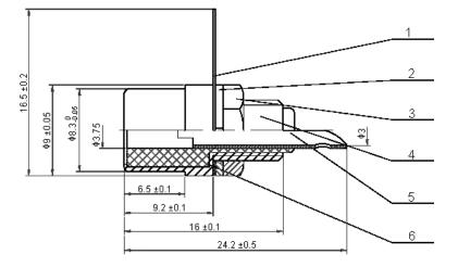
The female pin plating nickel, thickness 1µm (SOLDER).
