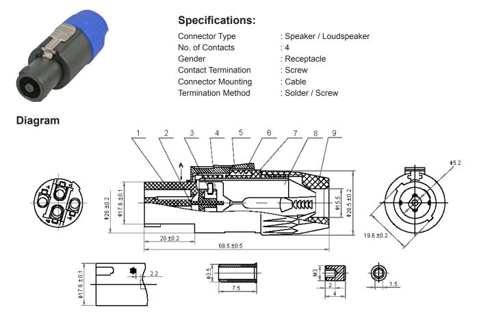
Pin with copper plating 10 $\mu$ m first, and then silver plating 4 $\mu$ m (SOLDER+SCREW).
