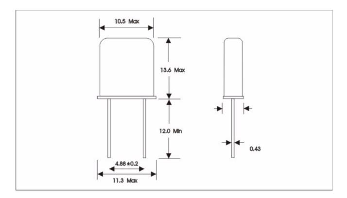
Holder Style Mode Adjustment Tolerance Temperature Stability Operating Temp. Range Load Capacitance ESR Marking HC-49/U Fundamental ± 30PPM at 25°C ± 50 PPM -20°C to +70°C 30 pF 40 Ohm Mark AELX027L\FREQ+WWYY
