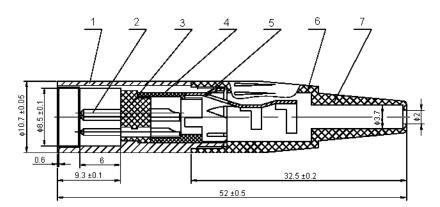
The pin plating gold, thickness 0.05µm (SOLDER).
