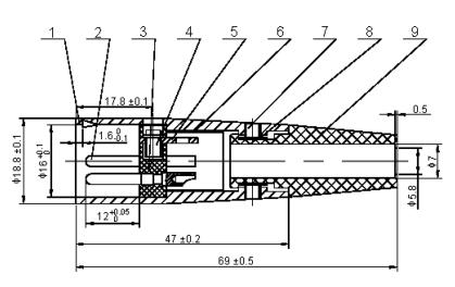
The pin plating silver, thickness 0.5µm (SOLDER).
