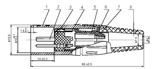
The pin plating silver, thickness 0.5µm (SOLDER).
