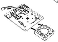
6. Route the wire neatly under the lugs on the fan support and connect the fan wiring to the two pin header on the PCB noting the polarity as shown.
