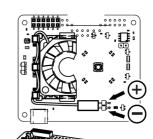
7. Clip the PCB onto the mounting pillars ensuring the riser pins locate through the holes in the board.
