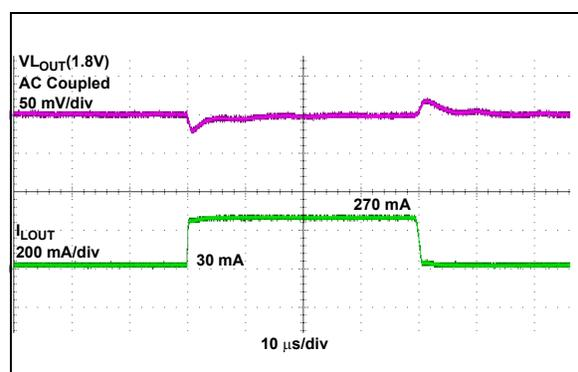
**FIGURE 2-18:** LDO Load Transient Response.
