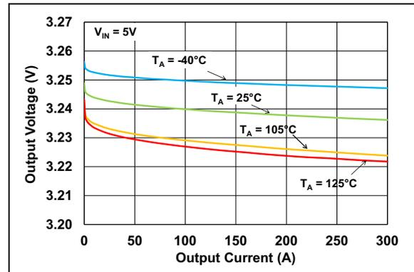
**FIGURE 2-10:** LDO Output Voltage vs. Output Current and Temperature (Load Regulation –  $V_{L\text{OUT}} = 3.3V$ ).
