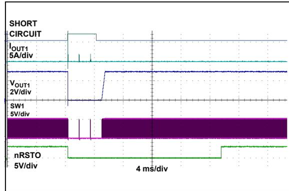
**FIGURE 2-17:** Output Short Circuit on  $V_{OUT1}$ .
