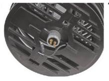
Pull the connector away from the pin and gently move to one side.
