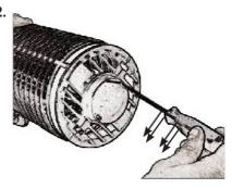
Remove the collection tray by squeezing the two recesses on the tray firmly and pulling the tray away. Note: Remove the tray over a rubbish bag to avoid dropping any insects. Release the clips of the lamp cover using a screwdriver. Pull the screwdriver in the direction indicated above.
