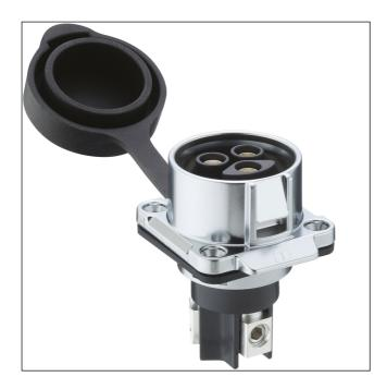
Quicklock flange chassis socket, IP67, size 28, straight version, with metal housing, screw clamps (8-pole version with solder terminals) and protecting cap (IP65)
