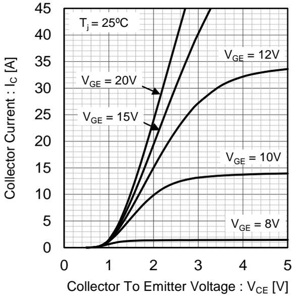
Fig.6 Typical Output Characteristics
