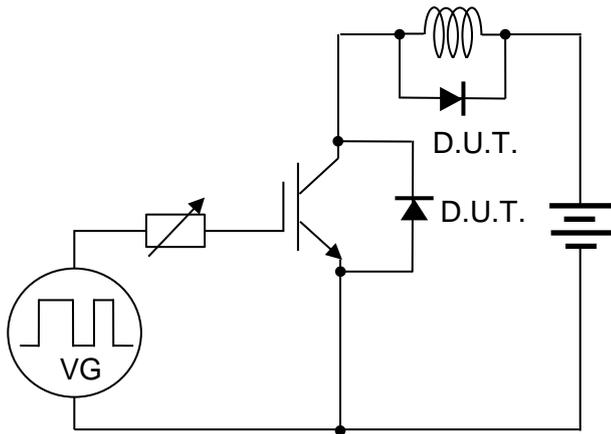
Fig.23 Inductive Load Circuit
