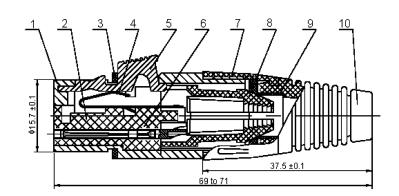
Female pin plating silver, thickness 0.5µm (Solder).
