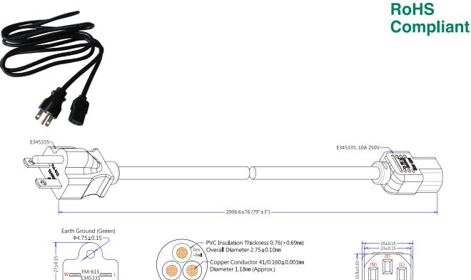
Blue Brown PVC Jacket Thickness 0.76mm(>0.61mm) Overall Diameter 7.8±0.2mm SJT 18AWGx3C (Wire Cross-Section) ME-302 (IEC 60320, C13, 10A 250V~) (Dimensions of Connector Face)
