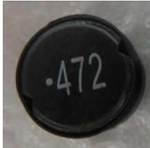
Marking with pad-printing
