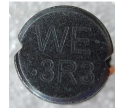
Marking with laser-printing (with WE logo)
