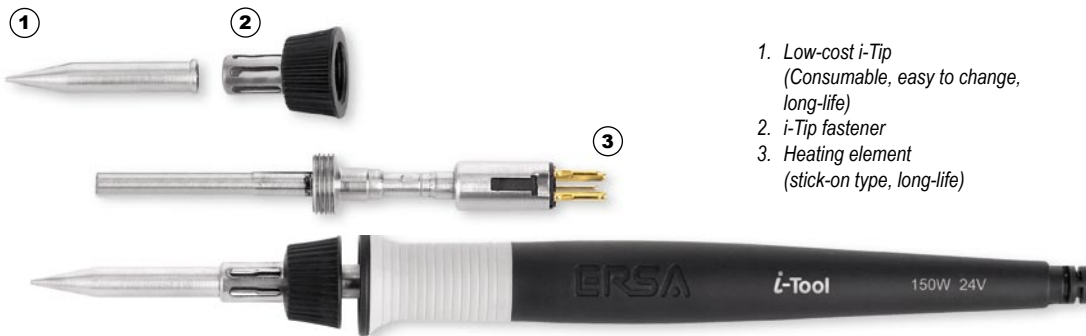
i-Tool soldering iron: ultra light (only 30 grams), ultra short (only 155 mm), and ultra short tip-to-grip (only 45 mm).
