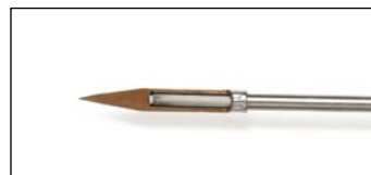
Cross-section of internally heated tip on the Micro tool SMD soldering iron with RESISTRONIC control
