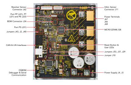
Figure 2: S12ZVM 3-phase motor control evaluation board description
