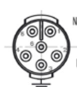
8MF1-PSM L: 85-264 VAC 4, 5, 6: Not connected
