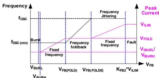
**Figure 4: Frequency and Peak Current vs. FB**
