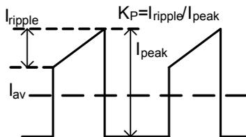
**Figure 11: Typical Primary Current Waveform**
