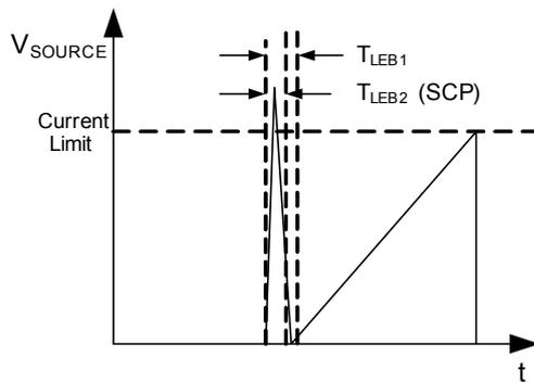
**Figure 10: Leading-Edge Blanking**
