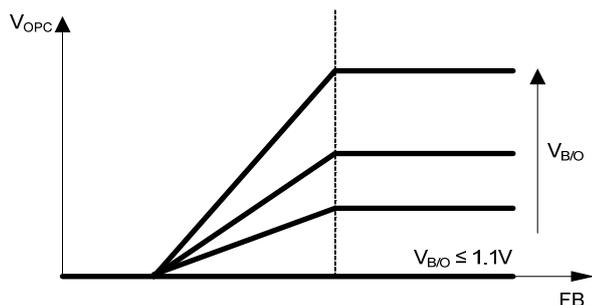
**Figure 9: Compensation Voltage vs. FB and B/O**
