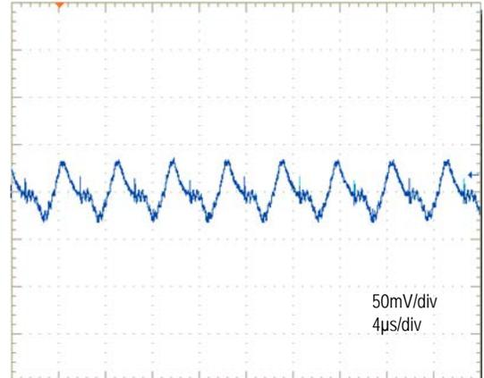
Transient Response ( $V_{in}=48\text{V}$ ,  $I_{out}=1.06\text{A}$  to  $2.125\text{A}$ ,  $T_a=+25^\circ\text{C}$ )
