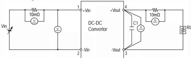
C1 : Ceramic Capacitor 0~400 $\mu$ F
