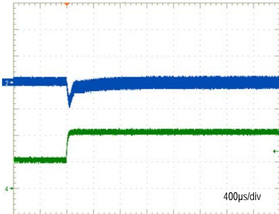
Transient Response ( $V_{in}=48\text{V}$ ,  $I_{out}=2.125\text{A}$  to  $1.06\text{A}$ ,  $T_a=+25^\circ\text{C}$ )
