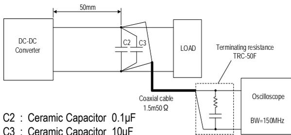
C2 : Ceramic Capacitor 0.1 $\mu$ F
