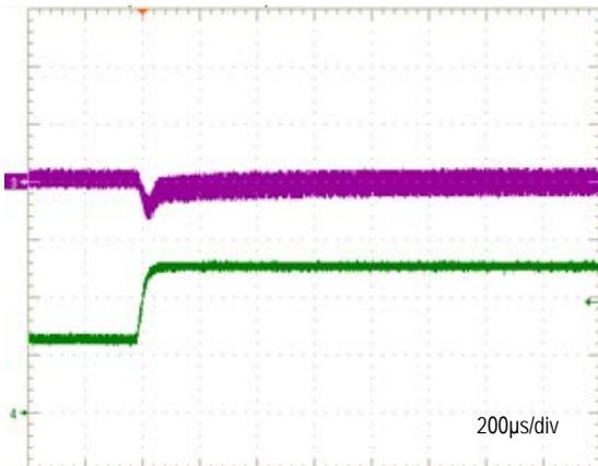
Transient Response (V<sub>in</sub>=48V, I<sub>out</sub>=2.55A to 5.1A, Ta=+25°C)
