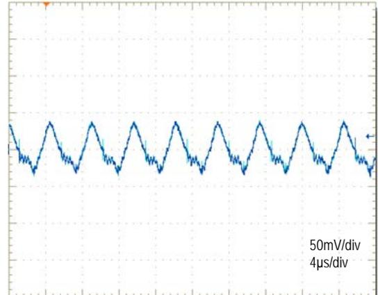
Transient Response (V<sub>in</sub>=48V, I<sub>out</sub>=2.55A to 5.1A, Ta=+25°C)
