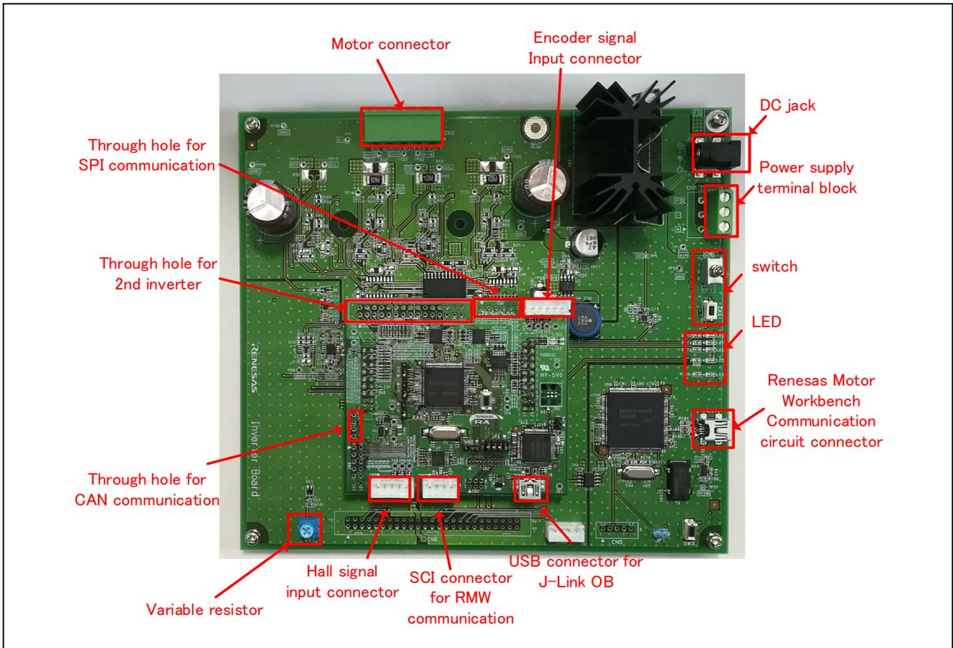
Figure 1-1 Main board (top view)
