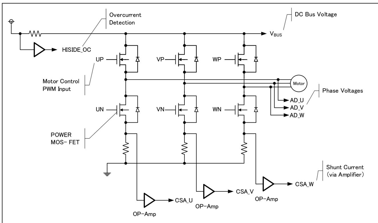
Figure 5-1 Illustration of inverter control circuit block
