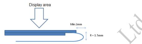
(12) The module should be fixed balanced into the housing, or the module may be twisted.
