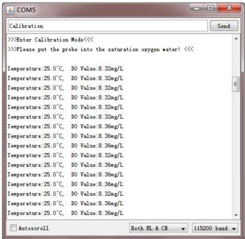
Enter "SATCAL" for dissolved oxygen calibration. The program will print whether the calibration is successful or not.
