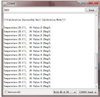
4. After the process stated above, the saturated dissolved oxygen calibration has completed. The probe is now ready for measurement.
