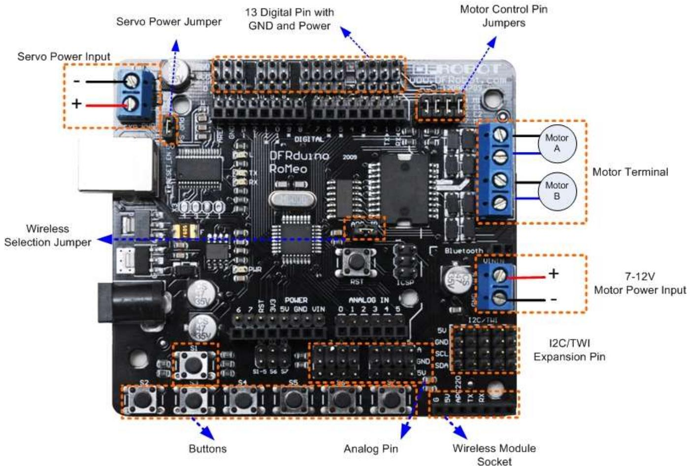
The picture above shows all of the I/O lines and Connectors on the Romeo, which includes:
