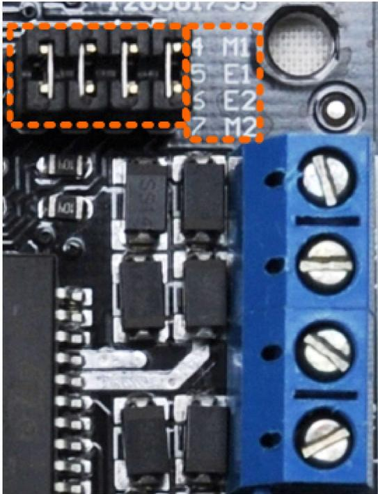
The PWM DC motor control is implemented by manipulating two digital IO pins and two PWM pins. As illustrated in the diagram above (Figure 5), Pin 4,7 (7,8 for old Romeo version) are motor direction control pins, Pin 5,6 (6,9 for old Romeo version) are motor speed control pins.
