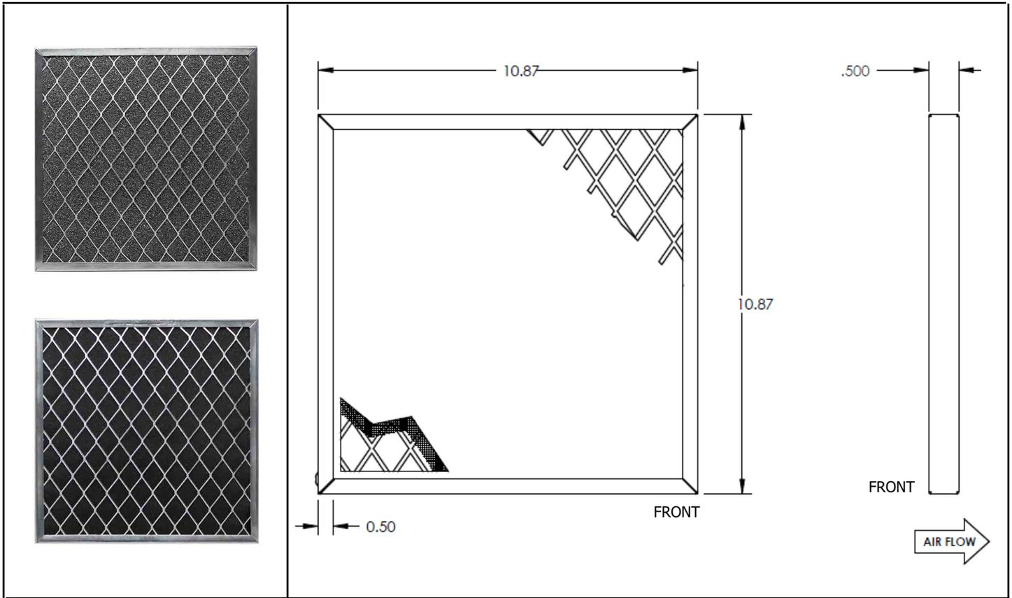
Orion Fans Hydrophobic Mesh air filters are water-repellent and offer a low pressure drop, cost-effective solution. The combination of hydrophobic mesh on the downstream side and high density foam on the upstream side offers a durable, cleanable, and moisture-resistant product. Designed for outdoor cabinets, process equipment applications requiring mist elimination, or other harsh environment installations.
