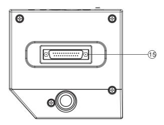
Trigger in connectorD-SUB pad signal input connector.
