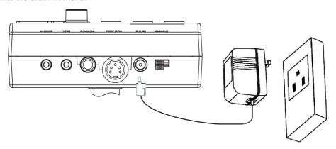
turn off the power switch before connecting with other devices.
