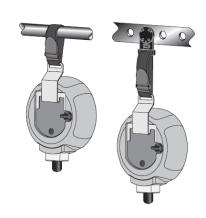
The FLUKE-GAUGEPAK is an easily installed hanging kit for the 700G Pressure Gauges. This accessory allows hands free pressure reading of the 700G gauge giving you the ability to perform addition functions such as pumping pressure, taking readings, and documenting test results. Installation of the GAUGEPAK is simple and provides the best angle position for best viewing of the gauge.
