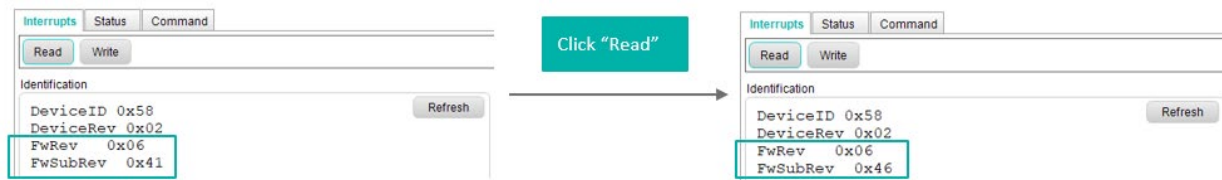
Figure 7. Firmware Version Readback
