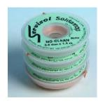
SOLDAMOP NO-CLEAN is manufactured using high purity oxygen free and oil free fine gauge copper wire. It is impregnated with a special 'No-Clean' flux. This flux significantly improves the wicking action of the braid. The residue left behind is halide free and nonconductive which means it does not need to be cleaned off
