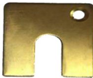
Short circuit metal sheet
