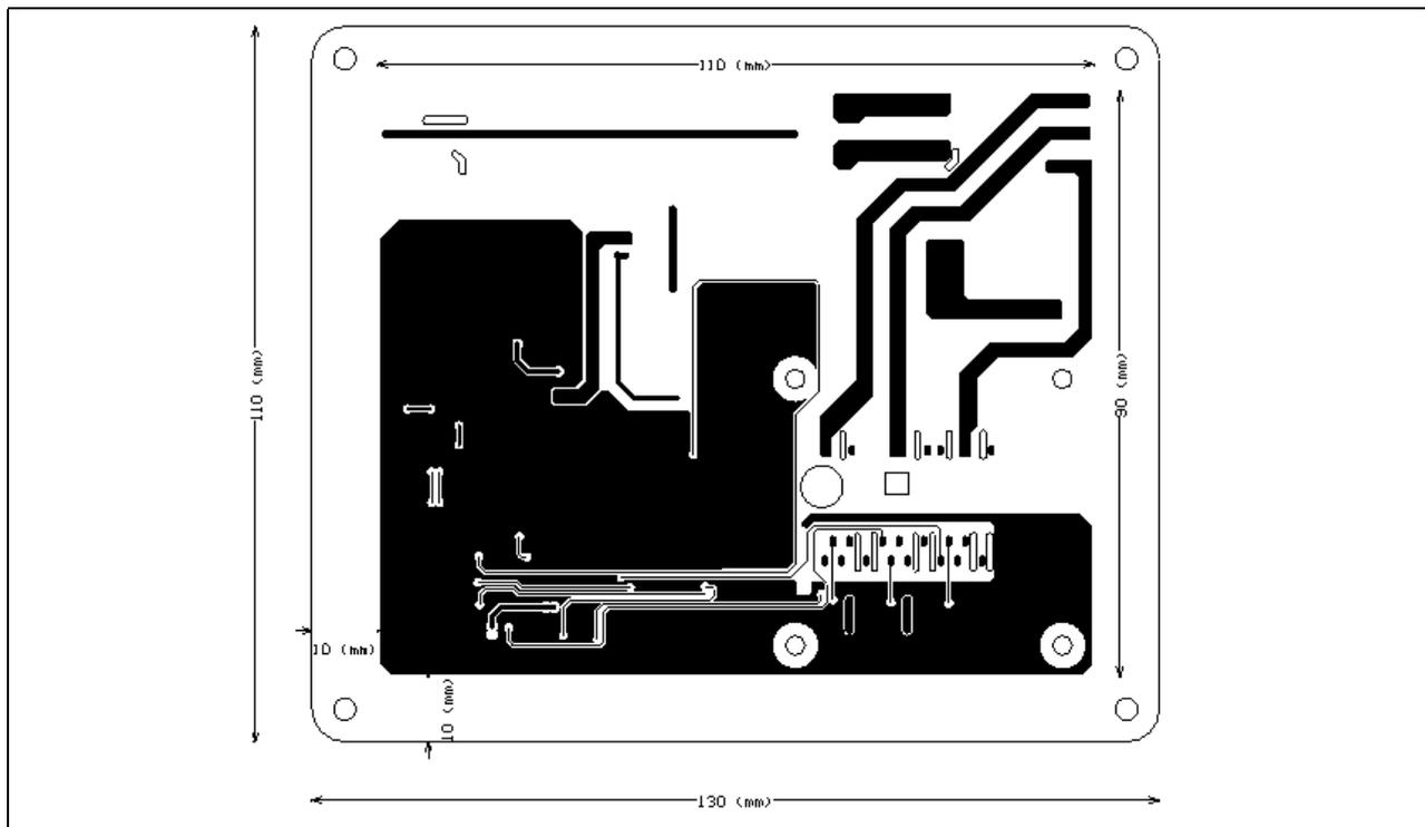
**Figure 21 Bottom layer routing of the EVAL-C101T-IM231**
