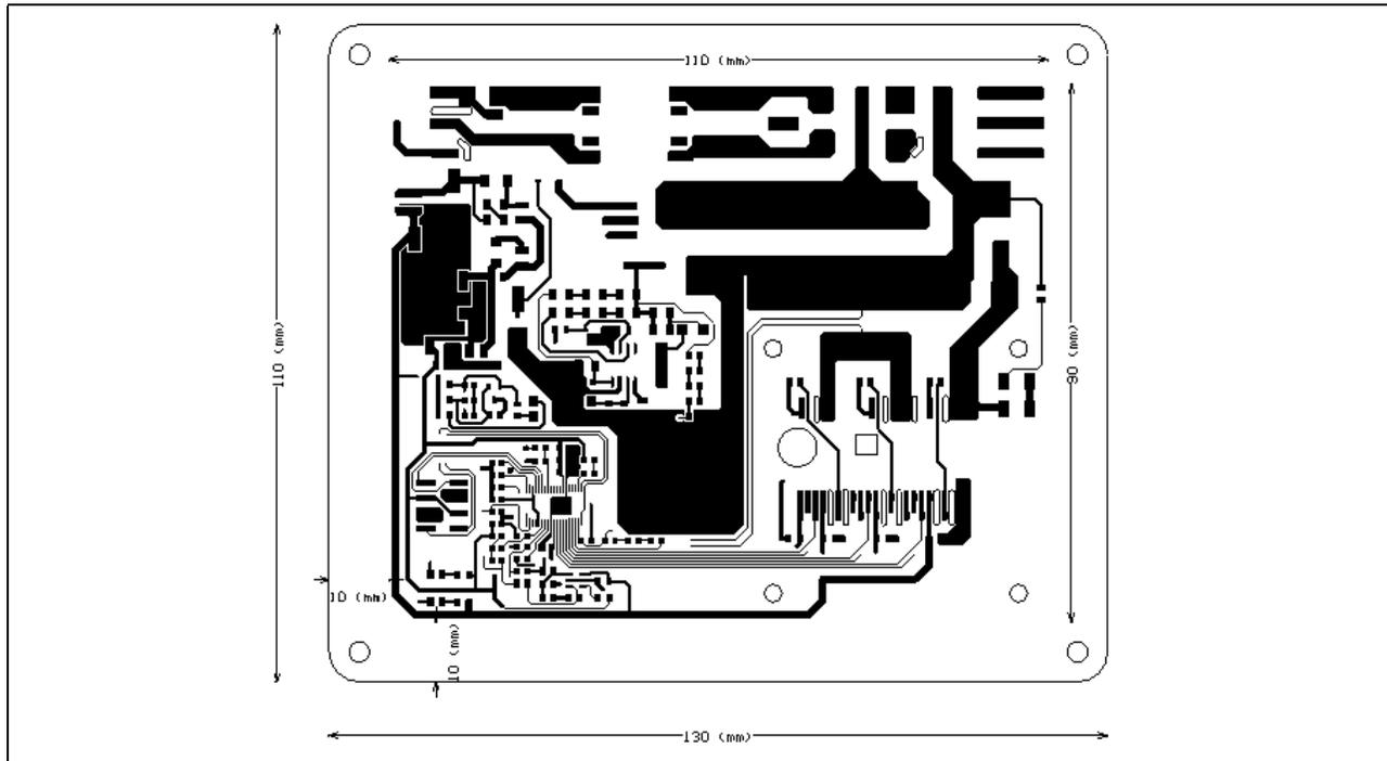
**Figure 20 Top layer routing of the EVAL-C101T-IM231**
