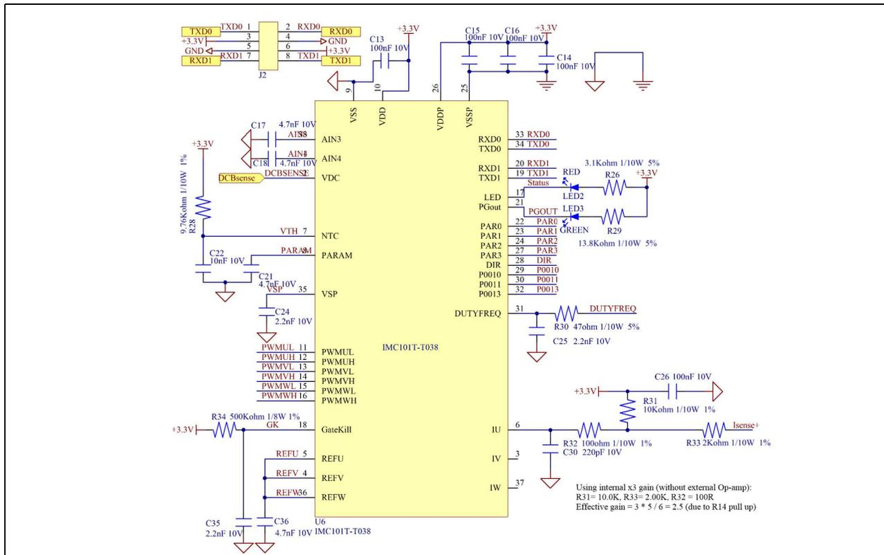
**Figure 15 The schematics for the EVAL-C101T-IM231 evaluation board**
