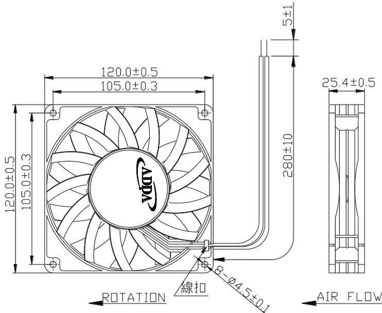
LEAD WIRES : UL 1007, AWG24 , L = 280±10 mm
