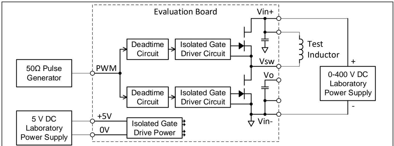
**Figure 2** Evaluation board typical application example (double-pulse test)
