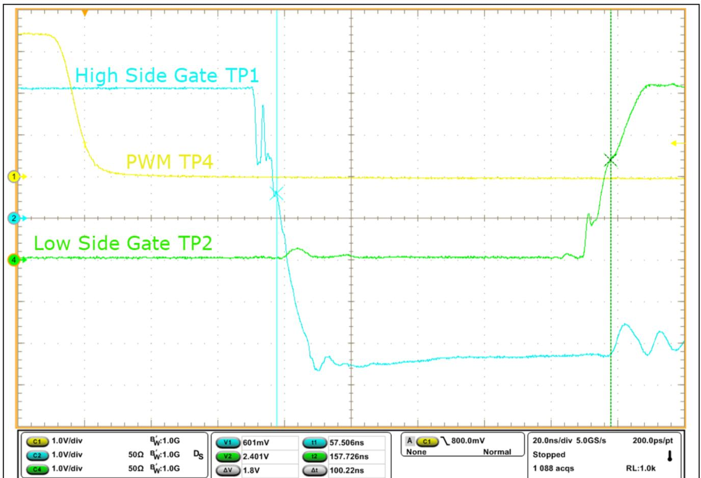
Figure 13 Measuring deadtime on the falling-edge of PWM
