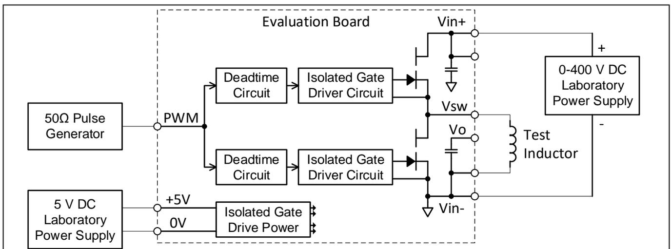
**Figure 3** Evaluation board connected for inverted double-pulse test
