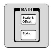
Note that Math and Limits are not available for Totalize. As shown in left diagram, the keys of 【Scale&Offset】 and 【Stats】 are included in MATH function area. The MATH function is disabled in the initial state and the annunicators of the two keys are OFF.
