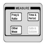
All measurement functions of this counter are included in the three keys. Use 【Freq&Ratio】 to measure the Frequency and Frequency Ratio of CH1 and CH2. Use 【 Time&Period 】 key to measure Period, pulse width(Postive or Negative) and time interval. And use
