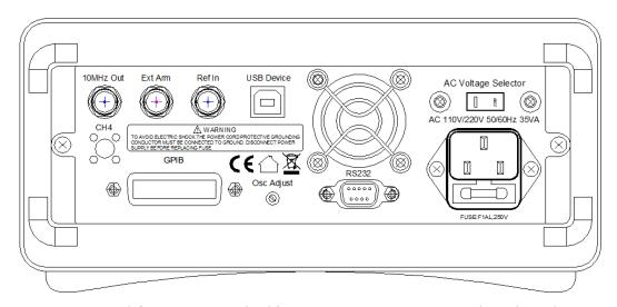
**Ref In** External frequency standard input, 5MHz or 10MHz can be selected, switch automatically inside the instrument.
