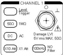
the trigger level and press 【Enter】 to confirm, and out of this function at present. Press this key again, the function is switched to polarity selection, 'SLOPE:POS' or 'SLOPE:NEG' will be shown in the display and the LED indicator will be on. Use 【 ↑ 】 【 ↓ 】 【 ← 】 【 → 】 key to select in the Positive and Negative, finally press 【Enter】 key to confirm.
